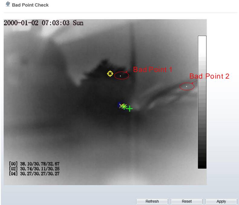
Figure 5-6 Bad point check interface
